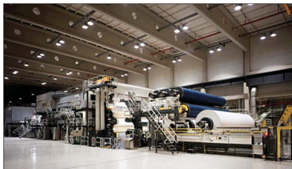
A modern paper-making machine can be as large as 33 feet wide, 66 feet high and the length of two football fields.
