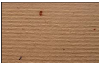
Uncoated paper with a laid finish and added flecks
